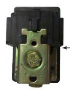
CUT-OUT PRESSURE SWITCH SETTING
